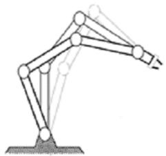
A robot arm is said to be redundant if *n*>*m*
